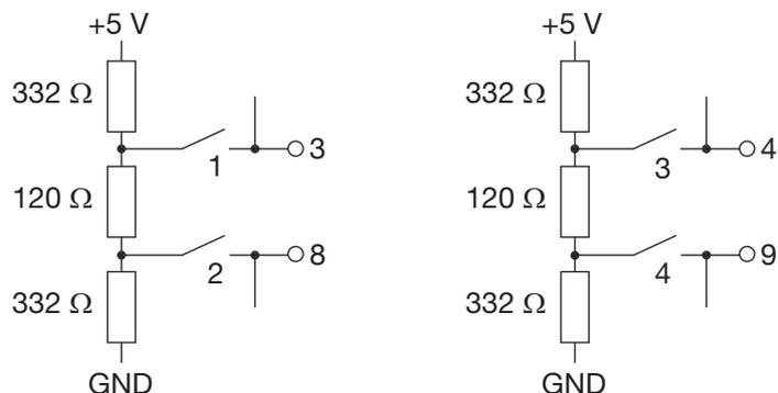
The terminating resistors are deactivated per default. To activate them, DIP switches 1 to 4 for the relevant interface must be pushed upward using a suitable tool such as a ballpoint pen (ON position).
